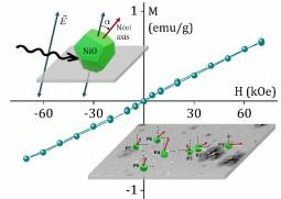
Figure 1: Magnetization curve at room temperature and distribution of Néel axes in a subset of single 34 nm NiO NP.
