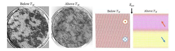
Figure 1: Left, XMCD images of the same area of permalloy on hematite below and above the Morin transition. The dichroic contrast is qualitatively different. Right, simulated images of the average ferromagnetic moment (below and above the Morin transition) after applying an external field. The circles and arrows show the direction of the Néel vectors of the underlying AFM layer (out- and in-plane, respectively).
