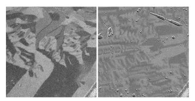
Fig 1. (Left) SPLEEM image, FOV 50μm, measure at room temperature. (Right). Same region and FOV taken at low temperature, after crossing the Verwey transition.
