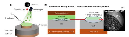
Figure 1: Scheme of the virtual electrode-LEEM approach to grow the Li/Na anodes (a), showing the profitable access to SSE/anode interface (b) and resulting XAS-PEEM image of the anode edge (c).
