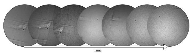
Figure 1: LEEM images of Ag time evolution during solid state dewetting process.
