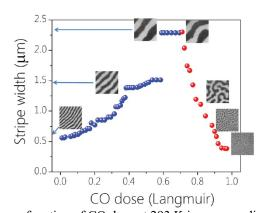
Figure 1: Magnetic domain width as a function of CO dose at 293 K in a perpendicularly magnetized Fe(2.4 ML)Ni(2 ML)/Cu(100) film. SPLEEM images with a field-of-view of 13 mm showing out-of-plane magnetic contrast at each stage of CO adsorption are included.
