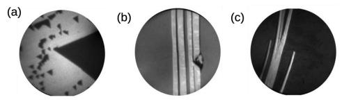
Figure: X-ray absorption images at (a) the  $M_5$  edge of Ba, the  $L_3$  edges of (b) Fe and (c) Mn of a BaWO<sub>4</sub> island and nanowires of FeWO<sub>4</sub> and MnWO<sub>4</sub>, respectively. The fields of view are 15  $\mu$ m, 10  $\mu$ m and 15  $\mu$ m.
