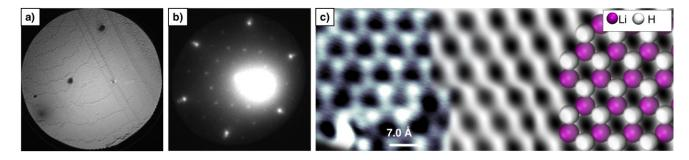
Figure 1. a) LEEM image with the clean terraces of the substrate of reference, the Au (111), with a FOV of 7  $\mu$ m b) LEED pattern of the structure of the lithium hydride 2D network taken at 35 eV c) Experimental (left) and DFT best-fit simulation (center) STM images (T = 77 K, I = 100 pA, V = -1.5 V) of the lithium hydride 2D network. Both images are merged in the central part. A schematic atomic model has been overlaid at the right part.
