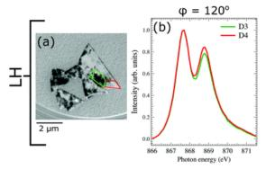
Fig. 1 (a) XMLD PEEM image of Fe-doped NiO triangles and (b) Ni L2 XAS microscpectra
